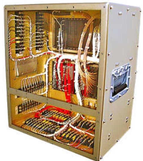
Inside view of Interchangeable Test Adaptor (ITA)
